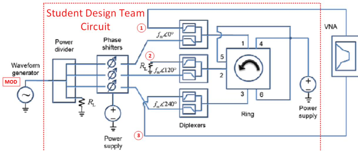
**Fig. 1.** Contest scheme for characterizing the insertion loss and nonreciprocal isolation parameters. In this picture, port 2 is terminated while the  $S_{31}$  parameter is measured. Details of *experimental setup* are discussed in *Supplementary Information* document of Estep, et al. *Nature Physics* **10.12**, 923-927 (2014).
