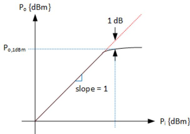
**Fig. 2.** Transfer function that will be used to determine  $P_{o,1dB}$  {dBm}.
